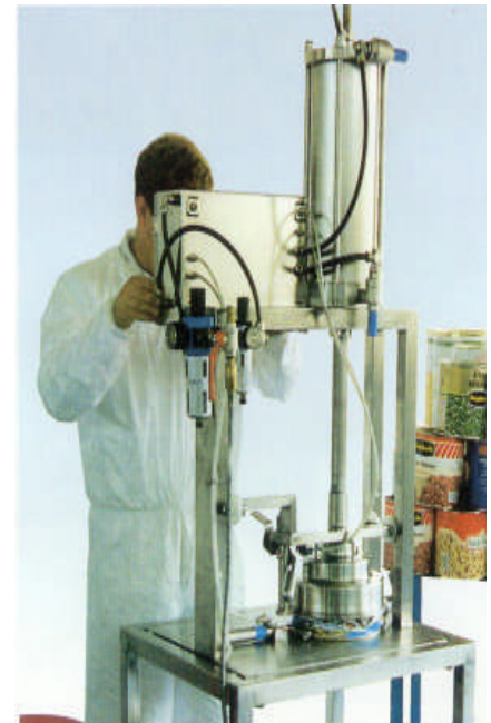
Compacting of the can and can lid
