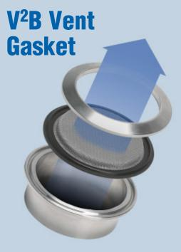
The Rubber Fab V2B Vent Gasket provides vacuum and pressure relief for **pharmaceutical** and **food/beverage processing** tank venting when **airborne particulate removal is required**. A 200 mesh screen combined with a 14 mesh screen of **sintered construction** creates a cost effective alternative to expensive vacuum breakers and venting systems.
