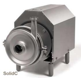
The SolidC pump series is a reliable and cost-effective solution for simple transport duties up to 85 m³/h. It utilizes the same mechanical shaft seal found in our LKH series, which is front-loaded and easily replaced without removing the backplate. SolidC pumps are available in four sizes and comply with 3A, CE and EHEDG requirements.
