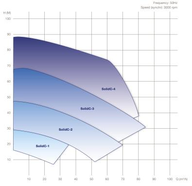
**SolidC performance** SolidC is a reliable, cost-effective centrifugal pump for standard duties up to 85 m<sup>3</sup>/h.
